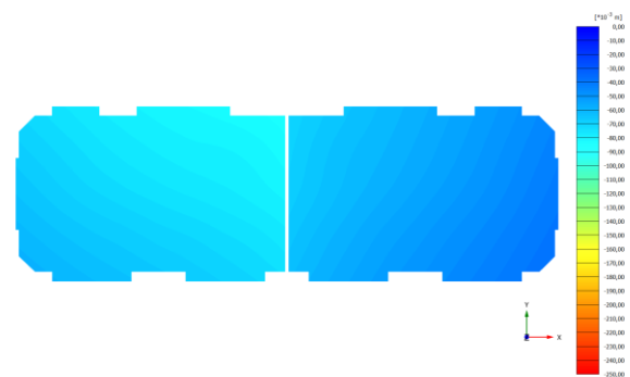
Total displacements u_x (scaled up 100 times) Maximum value = -0,03407 m (Element 108455 at Node 86) Minimum value = -0,07709 m (Element 108664 at Node 204)
