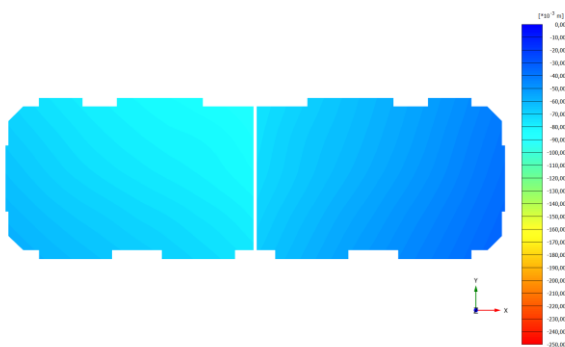
Total displacements u_x (scaled up 100 times) Maximum value = -0,03025 m (Element 108455 at Node 86) Minimum value = -0,08006 m (Element 108664 at Node 204)
