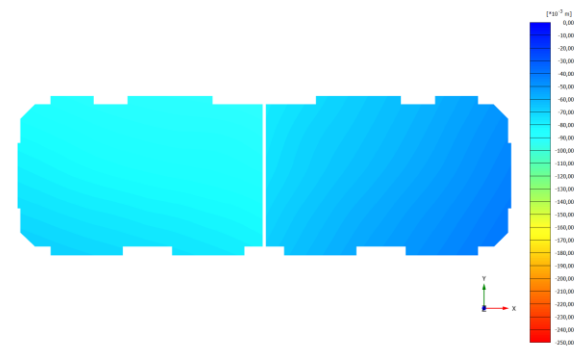
Total displacements u_x (scaled up 100 times) Maximum value = -0,03590 m (Element 108455 at Node 86) Minimum value = -0,08997 m (Element 108664 at Node 204)
