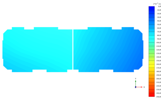
Total displacements u_x (scaled up 100 times) Maximum value = -0,03301 m (Element 108455 at Node 86) Minimum value = -0,09361 m (Element 108664 at Node 204)
