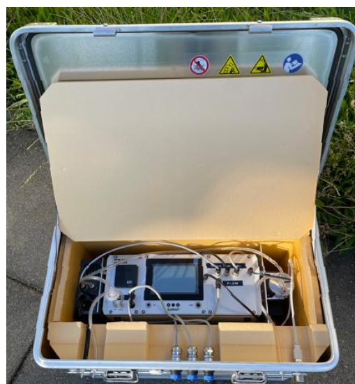
Fig.1. Thermal protection housing of the RTM2200 radon radiometer in an external aluminium casing. (Published with the kind permission of SARAD GmbH)
