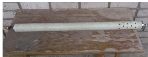
Fig. 4. The portable well sampler
